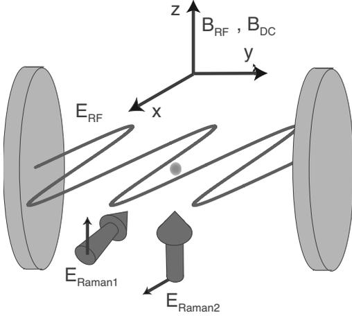
FIG. 2. Schematic setup of the proposed apparatus. The microwave cavity axis is along the  $y$  axis. The microwave electric field inside the cavity oscillates along the  $x$  axis. The two Raman laser beams are polarized along the  $x$  axis and  $z$  axis, respectively. The microwave magnetic field and the static magnetic field are both directed along the  $z$  axis. A dipole trap (not shown) holds the atoms at the origin that coincides with an antinode of the microwave electric field.
