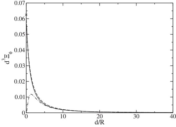
FIG. 4. Same as Fig. 2 but for the energy shift due to the  $\phi$  component of the atomic dipole. The solid line is the exact expression calculated numerically, the dot-dashed line is the  $m=1$  term alone, and the dashed line is the single integral derived through the uniform asymptotic approximation for the Bessel functions, Eq. (20b).
