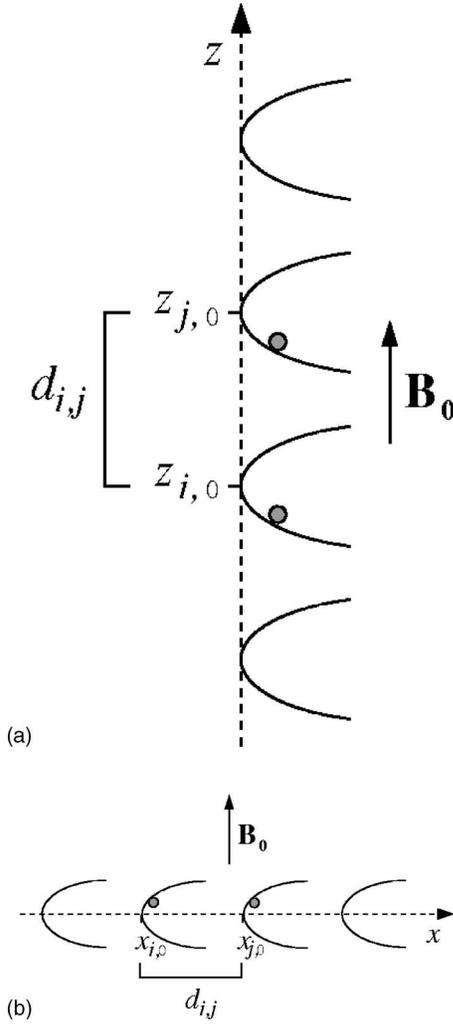
FIG. 1. Schematic drawing illustrating two different geometries for a linear array of micro-Penning traps. The traps are represented by sketching the electrostatic potential along the  $z$  axis. (a) The electrons are aligned along the  $z$  axis, parallel to the confining magnetic field; (b) the electrons are aligned along the  $x$  axis, orthogonal to the confining magnetic field.
