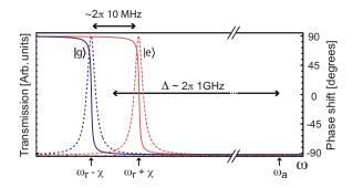
FIG. 2. (Color online) Resonator transmission (dashed lines) and corresponding phase shifts (full lines) for the two qubit states (blue: ground; red: excited). The numbers are calculated using  $g/2\pi\sim100$  MHz and  $g/\Delta\sim0.1$ . At the far detuned frequencies required for single qubit gates, the phase shift of the resonator field does not depend on the qubit state. In this case, there is negligible entanglement between the resonator and the qubit.
