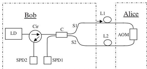
FIG. 1. Schematic diagram of the Sagnac QKD system employing an AOM-based phase modulator: LD—pulsed laser diode; Cir—circulator; C— $2 \times 2$  coupler; SPD1, SPD2—single photon detector.
