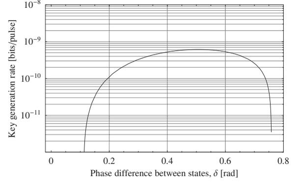
FIG. 8. Key generation rates at various distances. We use the QKD model parameters shown in Table I to compute the overall gain and the overall QBER from Eqs. (8) and (9). The key generation rates are then computed using Eq. (B14) with three  $B$  steps for various distances. Here, the key rates should be zero (since Eve launches an intercept-and-resend attack) but are positive in the range  $0.12 \leq \delta \leq 0.75$ , meaning that the keys generated in this range are insecure.
