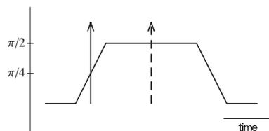
FIG. 3. The dashed line is the original signal pulse intended to be modulated at the middle of the phase modulator’s response to have a phase of  $\pi/2$ . Eve time shifts the pulse to the one in the solid line. This pulse now arrives at the middle of the rising edge and acquires a phase of  $\pi/4$  instead.
