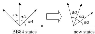
FIG. 2. The phase difference between the four states sent by Alice is changed by Eve to  $\delta$ . In standard BB84 states,  $\delta = \pi/2$ . (Note that the states are drawn so that orthogonal states are  $\pi/2$  apart in the diagram but are  $\pi$  apart in the actual phases.)
