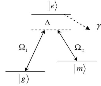
FIG. 3. Single-qubit rotation in two-photon Raman configuration. The detunings between two optical fields and the dipole transitions are large enough to cancel the excited state adiabatically.
