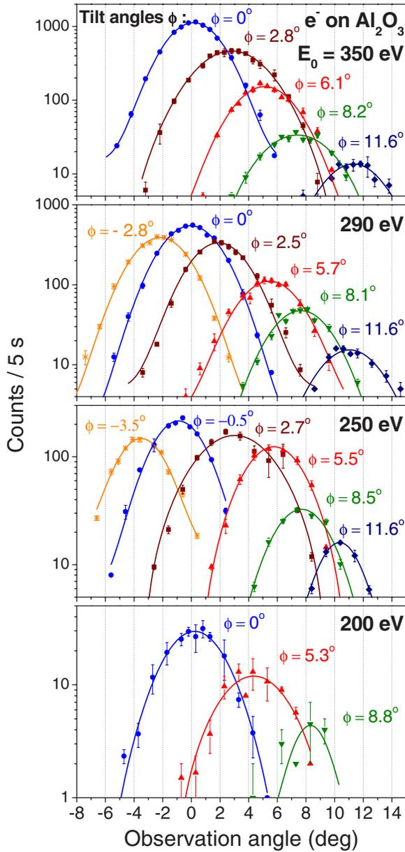
FIG. 2. (Color online) Angular distributions of electrons transmitted through the  $\text{Al}_2\text{O}_3$  nanocapillaries for different tilt angles ( $\phi$ ) and impact electron energies ( $E_0$ ).
