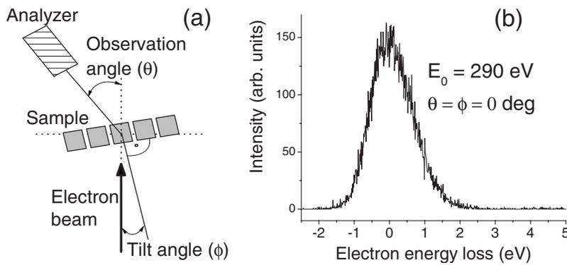
FIG. 1. (a) Definition of the observation ( $\theta$ ) and tilt ( $\phi$ ) angles. (b) The energy loss spectrum of transmitted electrons of 290 eV for  $\theta = \phi = 0^\circ$ .
