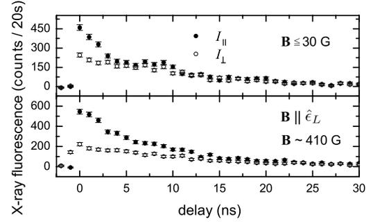
FIG. 3.  $\text{Kr}^+ 1s \rightarrow 4p$  resonance fluorescence as a function of laser/x-ray delay for low ( $< 30$  G) and high (410 G) magnetic fields. Target density,  $n = 2.3 \times 10^{15} / \text{cm}^3$ .
