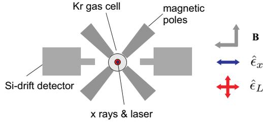
FIG. 1. (Color online) Experimental setup with magnetic field, laser, and x-ray orientations. X rays and laser copropagate into the plane of the page. For details see text.
