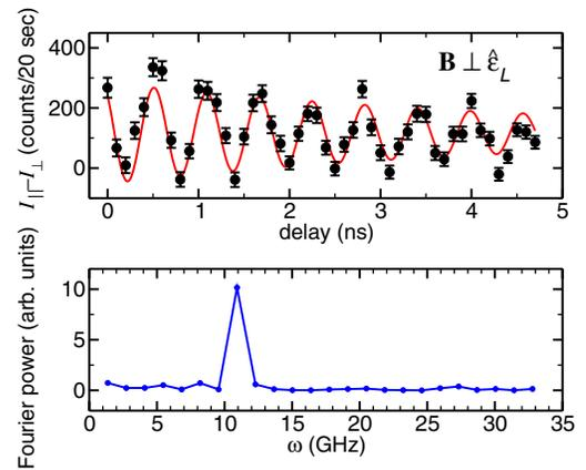
FIG. 4. (Color online) Top: Differential x-ray absorption ( $I_{\parallel} - I_{\perp}$ ) as a function of time delay for  $\mathbf{B} \perp \hat{\epsilon}_L$ . Bottom: Fourier transform of  $(I_{\parallel} - I_{\perp})$ . Target density,  $n = 2.3 \times 10^{15} / \text{cm}^3$ .
