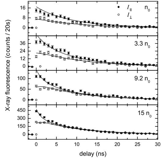
FIG. 2.  $\text{Kr}^+$  orbital alignment decay for various densities.  $\text{Kr}^+ 1s \rightarrow 4p$  resonance fluorescence versus laser/x-ray time delay for  $\hat{\epsilon}_L$  and  $\hat{\epsilon}_x$  parallel ( $I_{\parallel}$ ) and perpendicular ( $I_{\perp}$ ). Target density  $n_0=1.3 \times 10^{14} \text{ cm}^{-3}$ . Laser intensity is  $1.0(0.2) \times 10^{15} \text{ W/cm}^2$ . Solid curves were generated by theory.
