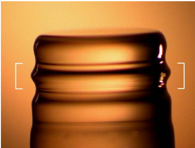
FIG. 1. (Color online) \text{CaF}_2 cavity with a record Q factor of (6.3 \pm 0.8) \times 10^{10} , 5.5 mm in diameter. White brackets show the area of WGM localization.
