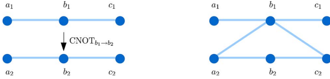
FIG. 2. (Color online) Effect of a CNOT gate on a product of two graph states. The final state is associated with a graph composed of the two initial graphs with additional edges between the control qubit b_1 and all neighbors of the target qubit b_2 .
