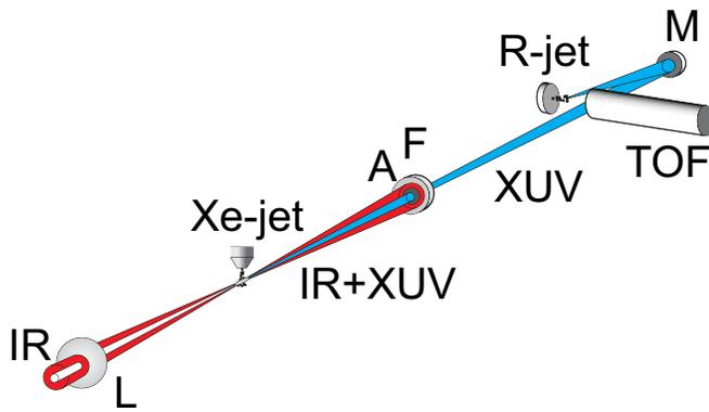
FIG. 1. (Color online) The experimental setup is shown. *L*: 3.5 m focal length lens; *A*: aperture; *F*: Sn filter; *M*: spherical mirror; *TOF*: time-of-flight spectrometer; *R*: face plate of the target jet serving as the extraction plate for the TOF spectrometer.
