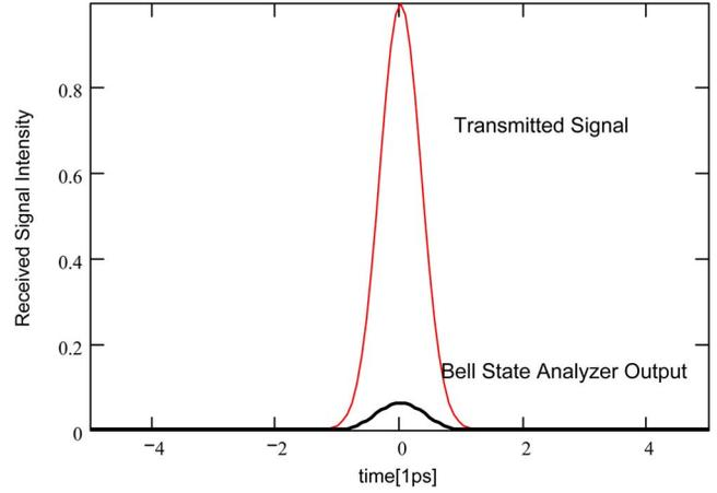
FIG. 3. (Color online) The output wave form of the bell state analyzer. For the Gauss wave form limiting filter with  $\sigma=3$  Thz at the transmitter, the intensity of the detection pulse  $D_4(t)$  of the bell state analyzer is degraded by 12 dB in intensity due to  $\bar{\alpha}_2=\bar{\beta}_2=\bar{\gamma}_2=1$  ps<sup>2</sup> and  $\bar{\alpha}_1=\bar{\beta}_1=\bar{\gamma}_1=1$  ps, but broadening of the pulse width is negligible.
