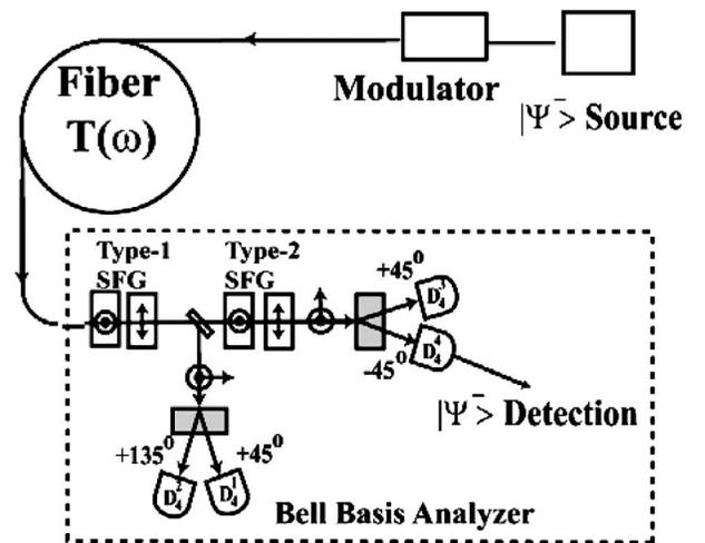
FIG. 1. Eigenstate  $\Psi^-$  optical fiber communication system.
