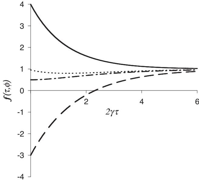
FIG. 2. Normalized conditional homodyne measurement  $f(\tau, \phi)$  as a function of  $2\gamma\tau$  for the ISHG with system parameters  $n_o=10^6$  and  $\bar{n}=0.2$  and phases  $\phi=0$  (solid line),  $\phi=11\pi/8$  (dotted line),  $\phi=\pi/4$  (dashed-dotted line), and  $\phi=\pi/2$  (dashed line).
