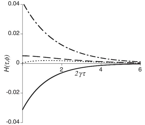
FIG. 5. Conditional homodyne measurement  $H(\tau, \phi)$  as a function of  $2\gamma\tau$  for the ISHG with system parameters  $n_o=10^6$  and  $\bar{n}=0.2$  and phases  $\phi=0$  (solid lines),  $\phi=11\pi/8$  (dotted lines),  $\phi=\pi/4$  (dashed lines), and  $\phi=\pi/2$  (dotted-dashed lines).
