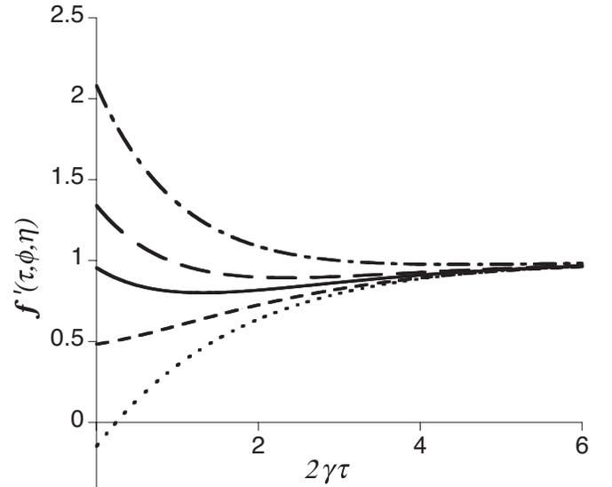
FIG. 3. Conditional homodyne measurement  $f'(\tau, 11\pi/48, \eta)$  as a function of  $2\gamma\tau$  for the ISHG with system parameters  $n_o=10^6$  and  $\bar{n}=0.2$  and error parameters  $\eta=-2 \times 10^{-4}$  (dotted lines),  $\eta=-5 \times 10^{-5}$  (dashed lines),  $\eta=4 \times 10^{-5}$  (long-dashed lines),  $\eta=2 \times 10^{-4}$  (dotted-dashed lines). The error-free measurement  $f(\tau, 11\pi/48)=f'(\tau, 11\pi/48, 0)$  (solid) is also shown for comparison.
