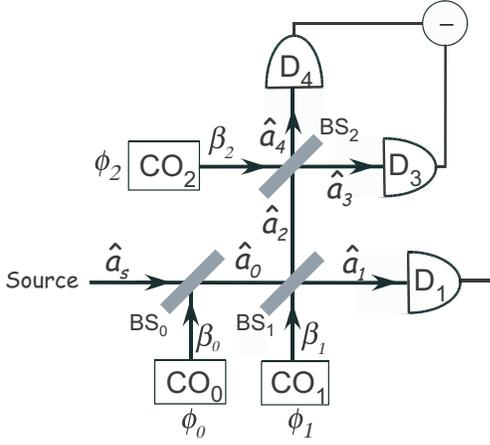
FIG. 1. (Color online) An outline of the setup for conditional measurement of quadrature fluctuations of a source  $\hat{a}_s$  with vanishing third-order field correlations.
