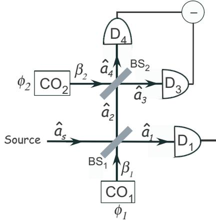
FIG. 4. (Color online) An outline of the setup for modified conditional measurement of quadrature fluctuations of a source  $\hat{a}_s$ .
