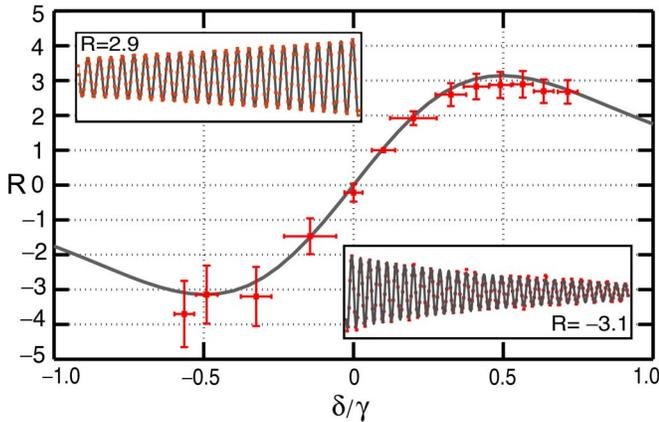
FIG. 3. (Color online) The instability measure  $R$  is plotted as a function of detuning of the cavity from resonance, for fixed input power. The solid (gray) curve is the theoretical prediction, given by a numerical solution to Eq. (1) with no free parameters. The squares show the measured data; the error bars are explained in the text. The inset time series show 3 s of data along with fits for the ringup and ringdown.
