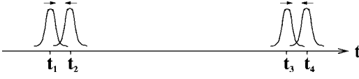
FIG. 1. Timing of the pulses. The counterpropagating pulse arrives with a time delay T=t_2-t_1 that is comparable to the pulse length \tau . The cycle may be repeated after T_c=t_3-t_1 > T, \tau .
