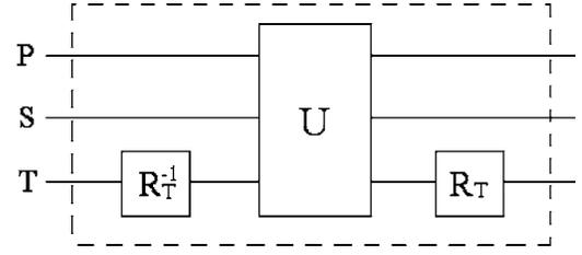
FIG. 3. The quantum circuit for realizing the Toffoli gate.  $U$  denotes the QPG with  $R_T$  being a single-qubit rotation.
