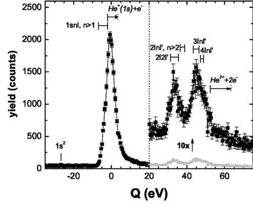
FIG. 2.  $Q$ -value spectrum of  $\text{Na}^{2+}$  recoils. The relevant He states are indicated, as well as the boundaries to transfer ionization ( $-2.0$  eV) and double ionization (52.4 eV). The arrows show the  $Q$ -value ranges in which transfer ionization or double ionization can be expected.
