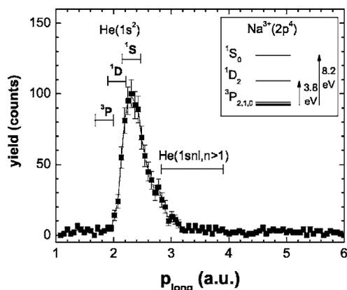
FIG. 3. A longitudinal momentum spectrum of Na<sup>3+</sup> recoils. The momentum resolution is 0.4 a.u. The assignment of the different target and projectile final states is explained in the text.
