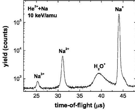
FIG. 1. A time-of-flight spectrum of recoil ions resulting from 10 keV/amu  $\text{He}^{2+} + \text{Na}(3s)$  collisions. Note that the presence of background  $\text{H}_2\text{O}^+$  recoils is enhanced because they are formed along the whole ion beam path ( $\sim 5$  cm), while the Na target has a diameter of about 1 mm only.
