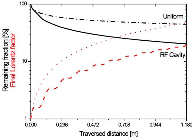
FIG. 2. (Color online) The surviving fraction of Ps<sup>-</sup> during acceleration in a  $E_0=60$  MV/m, 1269 MHz ( $\lambda=0.236$  m) rf cavity (solid line) with  $\phi=\pi/2$ , after acceleration in a 25-MV/m uniform field (dash-dotted line) and the respective Lorentz factors (rf, dashed line; uniform, dotted line), all as a function of cavity length.
