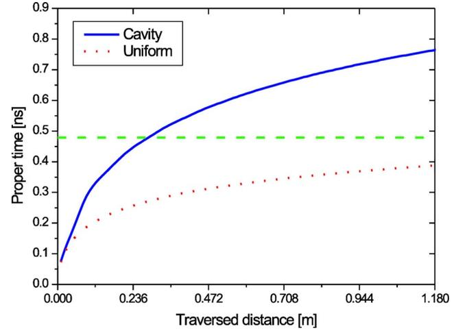
FIG. 1. (Color online) The proper time of  $\text{Ps}^-$  during acceleration in a  $E_0 = 60$  MV/m, 1269 MHz ( $\lambda = 0.236$  m) rf cavity (solid line) and in a uniform field of 25 MV/m (dotted line), both as a function of distance traversed. The horizontal dashed line shows the proper lifetime of  $\text{Ps}^-$ .
