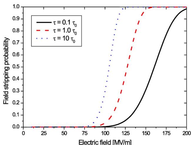
FIG. 4. (Color online) The field stripping probability as a function of electric field. The curves are calculated for  $\tau=0.1\tau_0$  ns (solid line),  $\tau=\tau_0$  ns (dashed line), and  $\tau=10\tau_0$  ns (dotted line).
