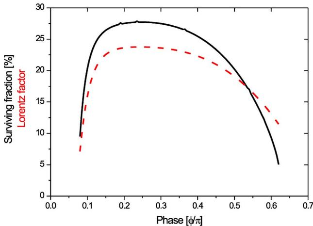
FIG. 3. (Color online) The surviving fraction (solid line) and the resulting Lorentz factor (dashed line) of Ps<sup>-</sup> after acceleration in a  $E_0=60$  MV/m, 1269 MHz ( $\lambda=0.236$  m) rf cavity as a function of phase.
