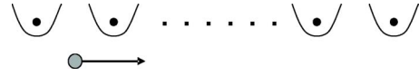
FIG. 1. Physical implementation of the repeated soft quantum measurements in an optical dipole trap: an atom, a carrier of quantum information, moves along the linear chain of atoms, which are located in the potential microtraps of the optical dipole trap, each of which performs a measurement.
