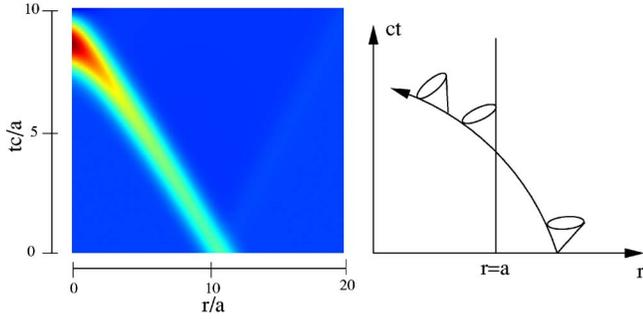
FIG. 1. (Color online) A density map of the real part of  $\psi_1$  in the  $r$ - $t$  plane (for the sake of clarity, the case of a quasilocalized wave packet at  $m=0$  is being shown). Due to the curved background, the wave-packet trajectory bends toward the sonic horizon at  $r=a$ . The light cone becomes parallel to the  $r=a$  axis, since no signal can escape from the horizon.
