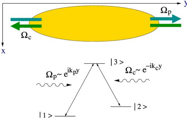
FIG. 1. (Color online) (top) Schematic representation of setup for light-induced effective magnetic fields: Two counterpropagating and overlapping laser beams interact with a cloud of cold atoms. (bottom) The level scheme for the  $\Lambda$ -type atoms interacting with the resonant probe and control beams characterized by Rabi frequencies  $\Omega_p$  and  $\Omega_c$ .
