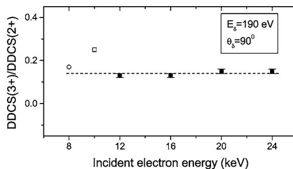
FIG. 3. Cross-section ratio  $\text{DDCS}(3+)/\text{DDCS}(2+)$  for production of triply and doubly charged argon ions corresponding to an ejected electron energy of 190 eV at  $\theta_\delta = 90^\circ$  vs incident electron energy. Present measurements:  $\blacksquare$ ; dashed line is the best fit to our data points; Hippler *et al.* (Ref. 11),  $\circ$  and Van der Wiel and Wiebes (Ref. 22),  $\square$ .
