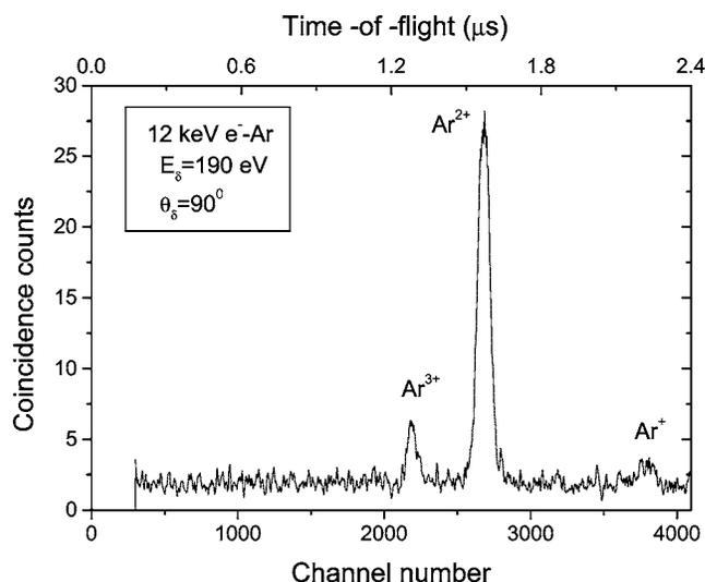
FIG. 1. Time of flight spectrum of argon ions produced from coincidences between the secondary electrons of 190 eV ejected at  $90^\circ$  and the recoil ions in collisions of 12 keV electrons with argon atoms.
