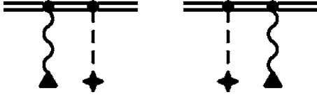
FIG. 1. Feynman diagrams for the lowest-order PNC transition amplitude. The wavy line terminated with a triangle indicates the absorbed photon. The dashed line terminated with a cross indicates the electron-nucleus weak interaction.
