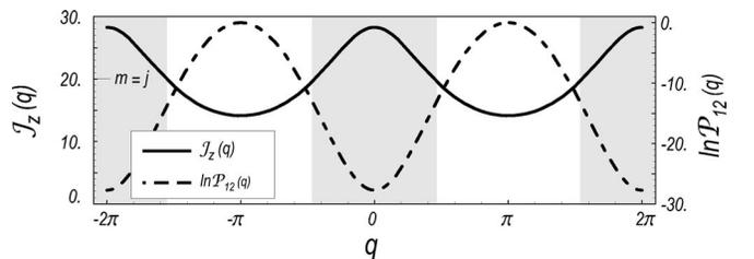
FIG. 4. Weak value  $\mathcal{J}_z(q)$  and log-likelihood  $\ln \mathcal{P}_{12}(q)$  for  $j=20$  and  $\hat{J}_z$  measurement with  $\mathbf{n}_1 = (0, 1/\sqrt{2}, 1/\sqrt{2})$  and  $\mathbf{n}_2 = (0, -1/\sqrt{2}, 1/\sqrt{2})$ , as depicted in Fig. 3. Shaded areas represent regions where the weak value lies outside the bounds of the spectrum  $[|\mathcal{J}_z(q)| > j]$ .
