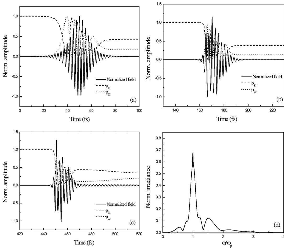
FIG. 5. (a)–(c)  $10\pi$ -pulse evolution at the respective distances of 0, 36, 120  $\mu\text{m}$  in our two-level-plus-continuum medium with  $\sigma^{(2)}=5 \times 10^{50} \text{cm}^4 \text{s}$ ; (d) the corresponding irradiance spectra at  $z=120 \mu\text{m}$ .
