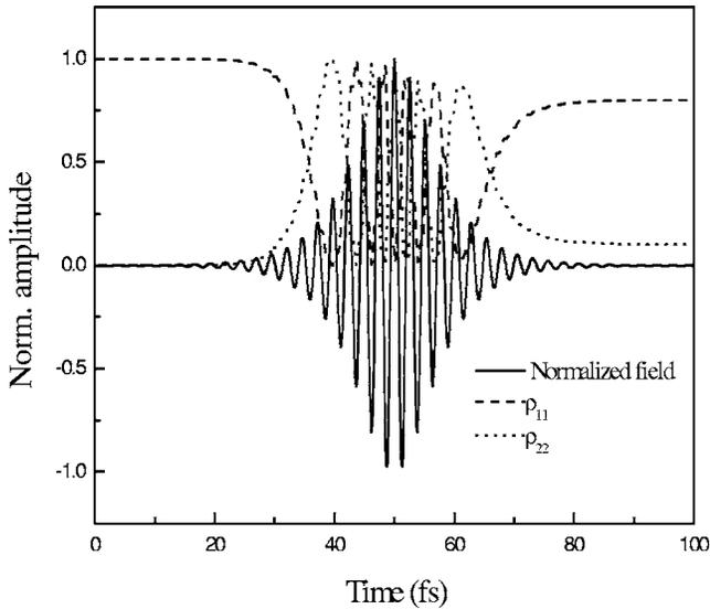
FIG. 2. The normalized electric field (solid line) and the population changes (dashed and dotted lines) near the input face of the two-level medium with  $\sigma^{(2)}=1 \times 10^{50} \text{ cm}^4 \text{ s}$ .
