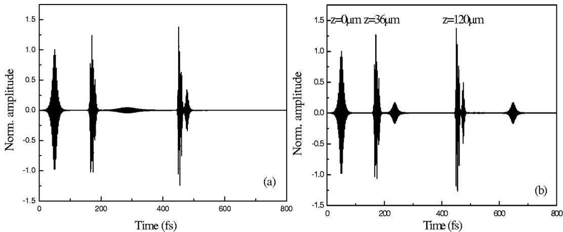
FIG. 3.  $10\pi$ -pulse evolution (a) in our two-level-plus-continuum medium with  $\sigma^{(2)}=1 \times 10^{50} \text{ cm}^4 \text{ s}$ ; (b) in a conventional two-level medium without ionization.
