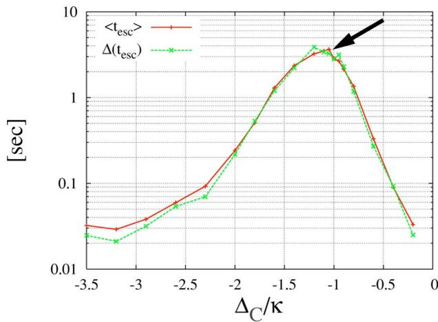
FIG. 2. (Color online) Trapping times as a function of the detuning of the field from the cavity resonance. Parameters are  $\Delta_A = -1000 \kappa$  and  $g = \kappa = \gamma/2$ , corresponding to the point indicated by the arrow in Fig. 1.  $P_e = 5\%$  on the whole range of  $\Delta_C$ .
