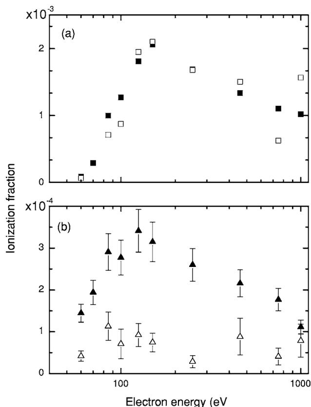
FIG. 4. Coincidence spectra from allene (solid points) and propyne (hollow points). (a)  $H^+ + C^+$  coincidences. (b)  $H^+ + CH_2^+$  coincidences. These spectra have been plotted as a fraction of the total target ion production at each energy. The  $H^+ + C^+$  spectra is a typical example of the coincidence spectra (including groups containing  $C_2$  and  $C_3$  chains) showing no difference between the isomeric molecules.
