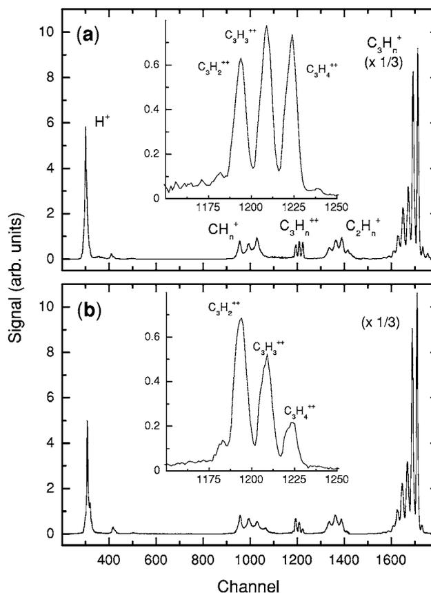
FIG. 2. Time-of-flight mass spectra taken for allene (a) and propyne (b) at 100 eV electron-impact energy. The insets show enlargement of the double-ionization groups,  $C_3H_n^{2+}$ .
