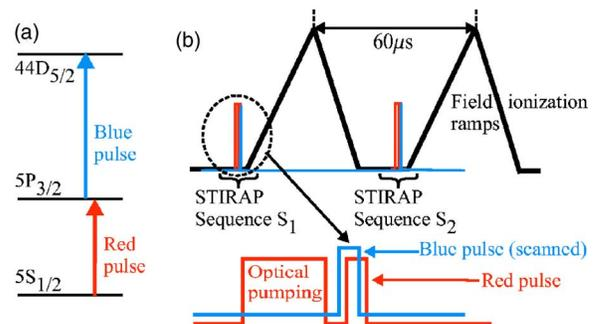
FIG. 1. (Color online) (a) Level diagram; (b) experimental timing diagram showing two STIRAP and field-ionization sequences. Two identical sequences,  $S_1$  and  $S_2$ , are required to provide a reliable measure of the excitation efficiency.
