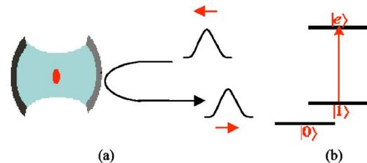
FIG. 1. (Color online) (a) Schematic setup for generation of cat states by reflecting a coherent optical pulse from a single-atom cavity. (b) The relevant level structure of the atom trapped in the cavity.
