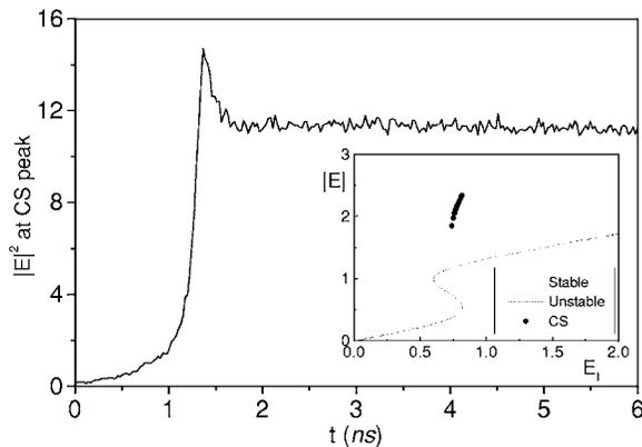
FIG. 4. CS switch-on process, numerical simulation. Parameters (in scaled units) are cavity detuning  $\theta=-2$ , normalized injected current  $J=2$  (laser threshold is  $J=2.11$ ), normalized WB amplitude  $E_{\text{WB}}=0.75$ , WB phase relative to the HB  $\phi=0$  rad. Small inset: homogeneous steady state (solid stable, dashed unstable) and CS as a function of the HB amplitude, for the parametric case in study. From now on, the HB amplitude is taken  $E_I=0.75$ .
