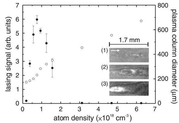
FIG. 3. Lasing intensity (solid circles) and the diameter of the plasma column produced by the pump pulse at 4 mm away from the entrance (open circles) as functions of average atom density. Inset shows interferograms of the plasma column taken at 50 ps after the pump pulse for (1)  $7.5 \times 10^{17}$ , (2)  $3.1 \times 10^{18}$ , and (3)  $6.2 \times 10^{18}$  cm<sup>-3</sup> atom densities. The pump pulse energy is 350 mJ, with no prepulse used.
