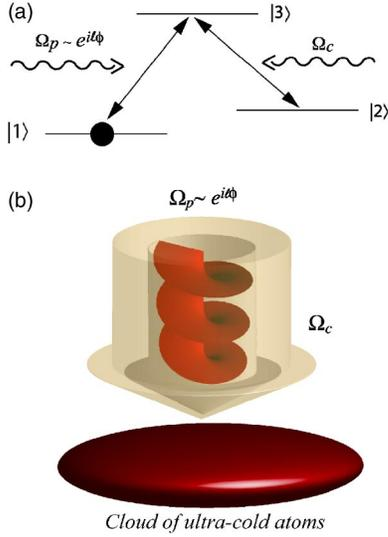
FIG. 1. (Color online) (a) The level scheme for the  $\Lambda$ -type atoms interacting with the resonant probe beam  $\Omega_p$  and control beam  $\Omega_c$ . (b) Schematic representation of the experimental setup with the two light beams incident on the cloud of atoms. The probe field is of the form  $\Omega_p \sim e^{i l \phi}$ , where each probe photon carries an orbital angular momentum  $\hbar l$  along the propagation axis  $z$ .
