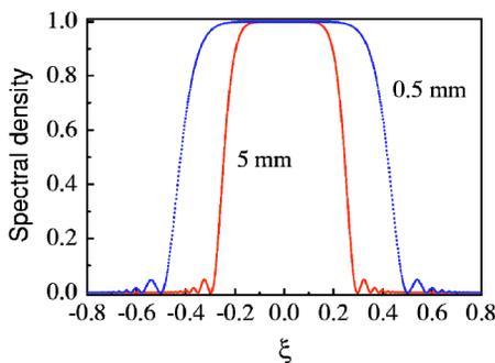
FIG. 2. Power spectrum of SPDC light vs frequency detuning for a 5-mm (inner curve) and 0.5-mm (outer curve)  $\text{BeSO}_4$  crystal at the crossover degenerate wavelength 923.8 nm.
