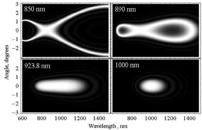
FIG. 3. SPDC spectra of a 5-mm  $\text{BeSO}_4$  crystal for different degenerate wavelengths. As expected, the “crossover” wavelength  $\lambda_0=923.8$  nm corresponds to the broadest spectrum of SPDC light irradiated in the forward (collinear with the pump) direction.
