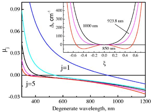
FIG. 1. The first five coefficients of the expansion (13) as functions of the degenerate wavelength  $\lambda_0=2\pi c/\omega_0$  calculated for the  $n_o$  in  $\text{BeSO}_4$  by differentiating the Sellmeier equation. Inset: The wave detuning  $\Delta_k(\nu)$  vs relative frequency detuning  $\xi$  for a 5-mm-long crystal.
