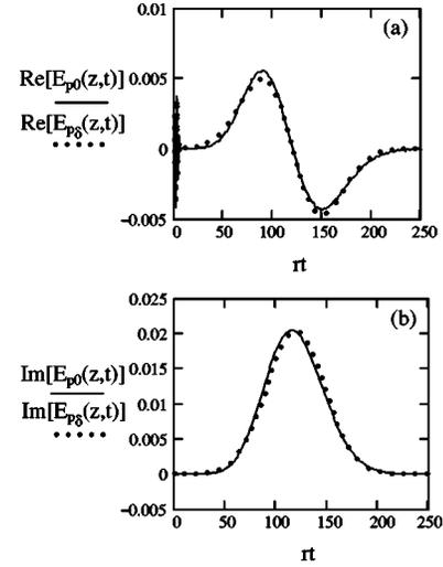
FIG. 8. Beat notes of the real (a) and imaginary (b) components of the probe pulse output for  $\delta t_{dA} = \pi/2$ . The thin solid line shows the numerical calculation of the integral (9) and the dots show the analytical approximation (55). The parameters are  $\gamma/\Gamma = 10^{-3}$ ,  $\Omega_d/\Gamma = 0.5$ ,  $r = \Gamma$ , and  $T = 30$ .
