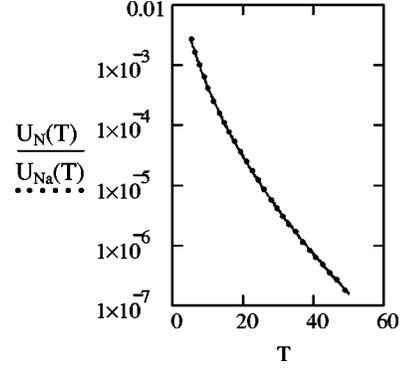
FIG. 11. Comparison of the numerically calculated integral (B2), solid line, with the analytical approximation (48), shown by dots. Both plots are normalized to  $U(0)$ . The parameters of the pulse and the sample are the same as for Fig. 6.  $T=\alpha z/\Gamma$  is the optical thickness of the absorber.
