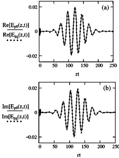
FIG. 9. Beat notes of the real (a) and imaginary (b) components of the probe pulse output for  $\delta t_{dA} = 10\pi$ . The thin solid line shows the numerical calculation of the integral (9) and the dots show the analytical approximation (55). The other parameters are the same as for Fig. 8.
