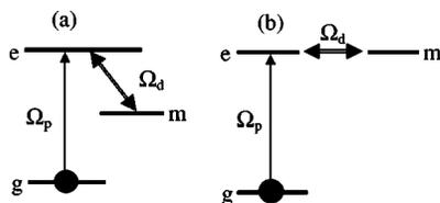
FIG. 1. Three-level atom excited by the probe  $\Omega_p$  and drive  $\Omega_d$  fields. The amplitude of the probe is time dependent and the amplitude of the drive is not.  $g$ ,  $e$ , and  $m$  are ground, excited, and metastable states. (a)  $e$  and  $m$  states have different energies. (b)  $e$  and  $m$  are degenerate states and the drive is a dc field.
