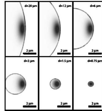
FIG. 3. Electric field profiles for a toroidal cavity with a principal diameter  $D=20 \mu\text{m}$  and minor diameters  $d=20, 12, 6, 3, 1.5,$  and  $0.75 \mu\text{m}$ . The calculations correspond to a TM-polarized mode near  $850 \text{ nm}$ . The optical mode behaves as a whispering-gallery-type mode until the minor diameter is below approximately  $1.5 \mu\text{m}$ , at which point the mode approaches that of a step-index optical fiber [28].
