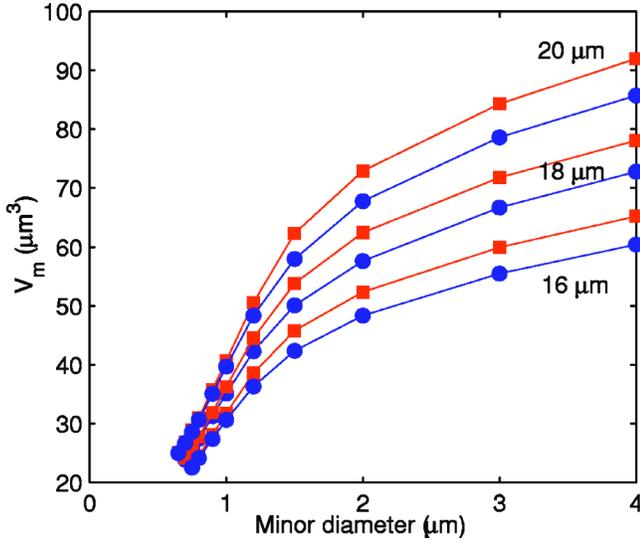
FIG. 4. Calculated mode volumes for a silica toroidal microresonator versus minor diameter for principal diameters of 20, 18, and 16  $\mu\text{m}$ . The plot shows both TM (squares) and TE (circles) polarizations. As the minor diameter is reduced a slow reduction of modal volume due to confinement in the azimuthal direction occurs, followed by a fast reduction for large confinement when the optical mode is strongly compressed in both the radial and azimuthal directions.
