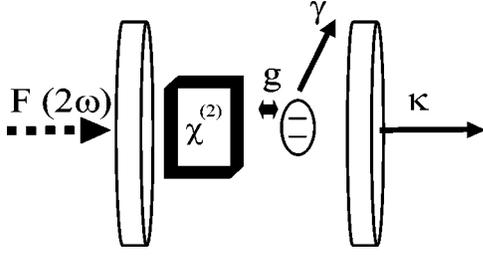
FIG. 1. Two-level atom inside a driven optical parametric oscillator.  $F^2$  is the input photon flux at frequency  $2\omega$ ,  $g$  is the atom-field coupling,  $\gamma$  is the spontaneous emission rate out the sides of the cavity, and  $2\kappa$  is the rate of intracavity intensity decay.
