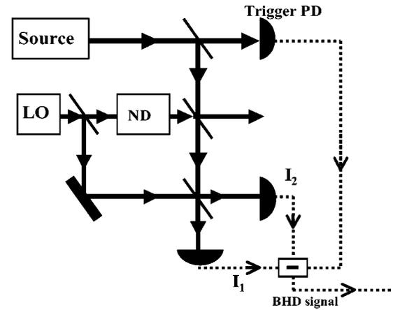
FIG. 2. A schematic of the measurement of  $h_\theta(\tau)$ . This is a balanced homodyne detection (BHD), conditioned on a trigger photodetection (PD). A part of the strong local oscillator (LO) is used as the offset field after adjusting the offset amplitude with a neutral density filter (ND)
