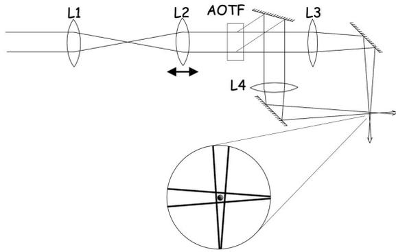
FIG. 1. Diagram of the optical system for the compressible crossed dipole trap. Computer-controlled translation of lens L2 changes the waist of the beams at their crossing point. The beams are divided and frequency shifted with an acousto-optic tunable filter (AOTF).
