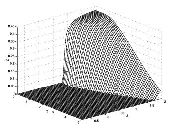
FIG. 6. The curved surface of thermal concurrence  $C_2$  between the next-nearest-neighbor sites as a function of the temperature and the next-nearest-neighbor interaction J. Here L=12.
