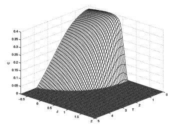
FIG. 5. The curved surface of thermal concurrence  $C_1$  between the nearest-neighbor sites as a function of the temperature and the next-nearest-neighbor interaction J. Here L=12.
