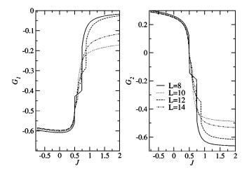
FIG. 1. The ground-state correlation function  $G_1$  (left) and  $G_2$  (right) versus *J* for various lattices. The singularity at J=1/2 arises from the level crossing (degeneracy).
