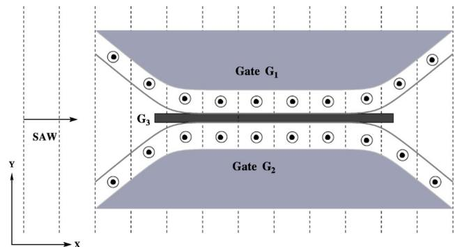
FIG. 1. Schematic plot of the SAW beam transporting electrons along a pair of channels. Two adjacent SAW dots in different channels form a pair of coupled quantum dots. The vertical lines in the figure represent maxima of the SAW potential which carries electrons (depicted as full circles) along the channels. The split gates defining the channels are denoted by  $G_1$ ,  $G_2$ , and  $G_3$ .
