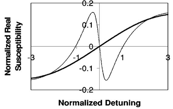
FIG. 3. Plot of the normalized real susceptibility  $\chi'_n$  as a function of the normalized detuning  $\delta_n$  for  $(\epsilon_v - \epsilon_{cd})/\epsilon_v = (\epsilon_v - \epsilon_{ac})/\epsilon_v = 0.5$ ,  $(\epsilon_{ab} - \epsilon_c)/\epsilon_c = 0.2$ , and  $\Omega_n = 1.8$ . The thick and thin solid lines correspond to  $\gamma_c/\gamma_a = 1$  and  $\gamma_c/\gamma_a = 10^{-3}$ , respectively.
