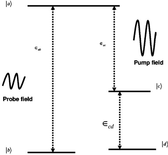
FIG. 1. Level scheme of a four-level atom. Quantum interference is introduced by driving levels  $|a\rangle$  and  $|c\rangle$  with a strong pump laser field and levels  $|a\rangle$  and  $|b\rangle$  by a probe laser field. The levels  $|a\rangle$  and  $|c\rangle$  decay to levels  $|c\rangle$  and  $|d\rangle$ , respectively.
