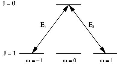
FIG. 1. The  $J=1-J=0$  atomic system interacting with two circularly polarized laser beams.
