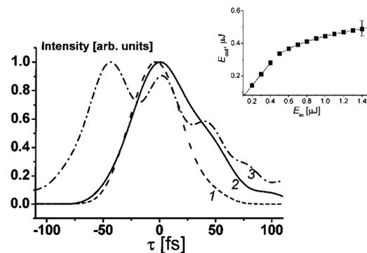
FIG. 6. The envelopes of laser pulses transmitted through the hollow PCF in the fundamental air-guided mode. The input pulse energy is (1) 0.1, (2) 1.4, and (3)  $3 \mu\text{J}$ . The inset shows the output energy measured as a function of the input energy for the fundamental mode of the PCF.
