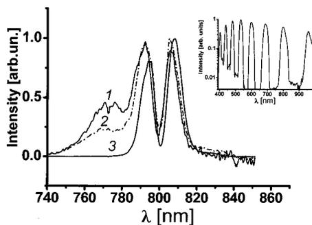
FIG. 5. Spectra of Ti:sapphire laser pulses transmitted through the hollow PCF in the fundamental (1) and higher order (2,3) air-guided modes. The inset shows the transmission spectrum of the fiber.
