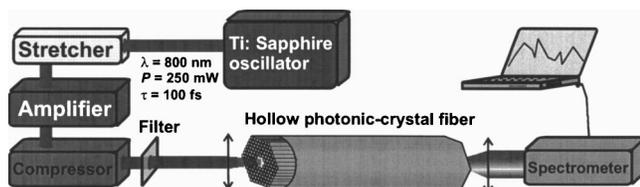
FIG. 3. The laser setup for the investigation of transmission and self-phase modulation of femtosecond laser pulses in a photonic-crystal fiber.
