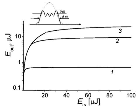
FIG. 1. The energy  $E_{\text{out}}$  at the output of a hollow photonic-crystal fiber calculated with the use of Eqs. (4) and (5) as a function of the input energy  $E_{\text{in}}$  for  $E_{\text{lim}}=0.65 \mu\text{J}$  (1),  $10 \mu\text{J}$  (2), and  $50 \mu\text{J}$  (3). The inset sketches the spectrum of an SPM-broadened laser pulse with a bandwidth  $\Delta\omega$  against the PCF passband with a width  $\delta\omega$ .
