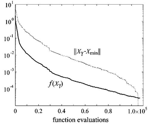
FIG. 4. Convergence of the algorithm for the Fredkin gate. The error function values are indicated by the solid line and the distance of the parameter sequence from the numerical optimum  $X_{\min}$  by the dotted line.
