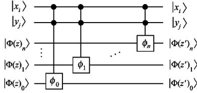
FIG. 12. Quantum circuit for the twice controlled addition of a classical number  $b$  into the quantum register  $|z\rangle_{n+1}$  in the Fourier basis. The twice controlled phase-shift gates serve to yield the phase shift  $e^{2\pi i \phi_k/2^n}$  provided that the control qubits  $|x_i\rangle$  and  $|y_j\rangle$  are active.
