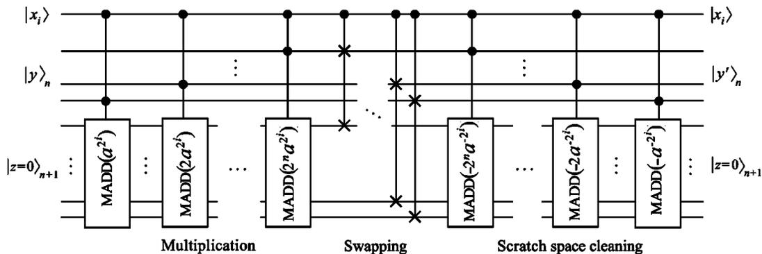
FIG. 9. Decomposition of the  $cMMUL(a^{2^i})$  gate using  $c^2MADD(b)$  and controlled swap gates. If the controlling qubit  $|x_i\rangle$  is active the resulting state is  $y' \equiv y + a^{2^i} \pmod N$ , otherwise  $y' = y$ . Note that the gate utilizes an additional ancilla register  $|z\rangle_{n+1}$  to perform the calculation.
