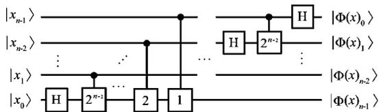
FIG. 11. Quantum circuit for an  $n$ -qubit Fourier transformation. Here  $H$  stands for the Hadamard gate. The controlled phase-shift gates are labeled with the numbers  $k$  which correspond to the phase shifts  $e^{i2\pi k/2^n}$ . Note the reversed order of the qubits on the right-hand side.
