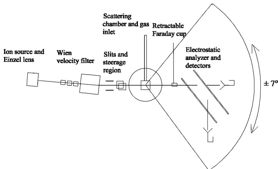
FIG. 1. Schematic diagram of the experimental apparatus.
