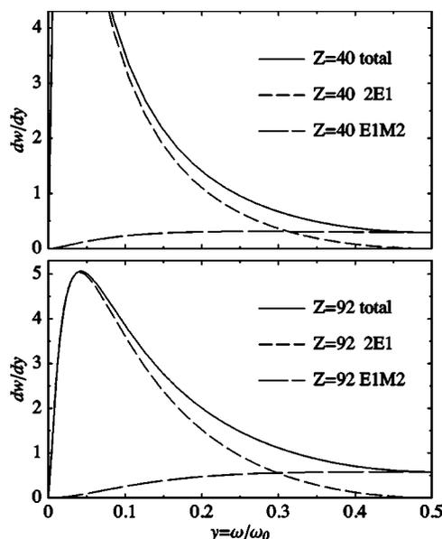
FIG. 3. Lower energy part of the spectral distributions of the  $2E1$  and  $E1M2$  contributions to the He-like  $2^3S_1$  two-photon decay rate as a function of the fractional energy  $y = \omega/\omega_0$ . (Present calculation in length gauge.) The sum of the two contributions (total) is also given. The upper plot is for  $Z=40$  and lower plot is for  $Z=92$ . All curves are normalized to area (=2 for the “total” curves over  $y=0 \rightarrow 1$ ).
