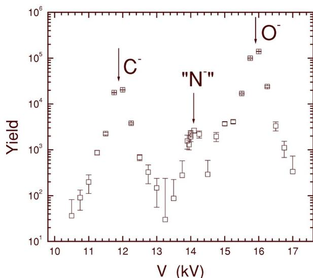
FIG. 1. The intensity of  $C^-$ , apparent  $N^-$  (denoted as  $N^-$  in the figure), and  $O^-$  ions detected by the narrowly collimated detector as a function of the deflector voltage.
