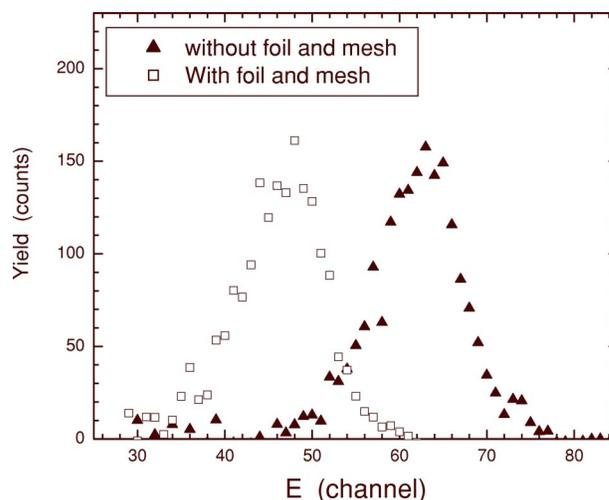
FIG. 2. The energy spectra of negative ions on the expected  $N^-$  trajectory with (open squares) and without (triangles) foil and mesh. Note that only a shift to lower energy as expected for an atomic ion can be seen.
