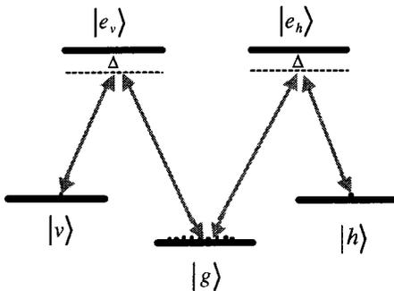
FIG. 1. The relevant-type double- $\Lambda$ -level structure of the alkali atoms in the ensembles. The metastable lower states  $|g\rangle$ ,  $|h\rangle$ , and  $|v\rangle$  can be achieved by, for example, Zeeman sublevels of electronic ground states  $5S_{1/2}$   $^{87}\text{Rb}$  atoms, and  $|e_h\rangle$  and  $|e_v\rangle$  ( $5P_{1/2}$ ) are the excited states.
