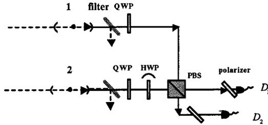
FIG. 2. We consider a setup in which individual atoms are trapped inside two spatially separated optical cavities 1 and 2. The atoms are illuminated by the synchronized pumping laser pulses and the forward-scattering Stokes pulses can leak out the cavities and are collected in the beam splitter after the filters. The dashed line represents the pumping laser pulses with the frequency  $\omega_l$  and the solid line represents the Stokes pulses.
