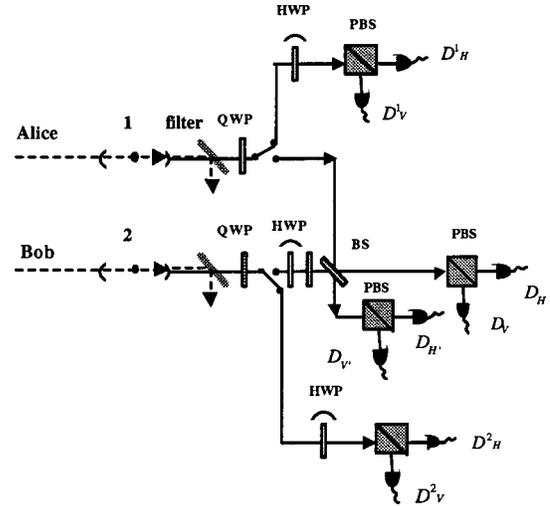
FIG. 3. Schematic setup for the realization of the secure direct communication between two users. In each station, there is a device called "space optical switch" which causes the photons to be sent to the proper mode via fiber. The dashed line represents the repumping laser pulses with the frequency  $\omega_o$  and the solid line represents the forward-scattering Stokes pulses.
