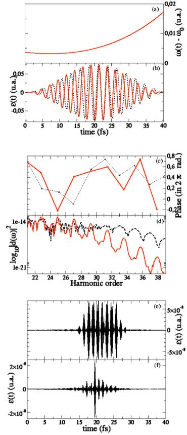
FIG. 2. Optimized emitted pulse using direct criterion  $J_2$  in a full 3D model: (a) the chirped function; (b) the excitation laser (dotted line, without chirp; solid line, with chirp) with a duration of 16 cycles; (c) phases calculated at the spectrum peaks; and (d) amplitudes of the HHOG spectrum (dotted line, without chirp; solid line, with chirp); (e) and (f) emitted laser pulse without and with optimization, respectively.
