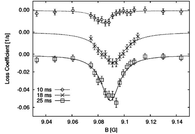
FIG. 2. Loss coefficients for a mixture of  $|2, -1\rangle$  and  $|1, +1\rangle$  states as a function of the magnetic field for hold times of 10, 18, and 25 ms. The loss coefficient is proportional to the two-body loss rate  $\bar{\gamma}$  multiplied by the hold time (see text for further explanation).
