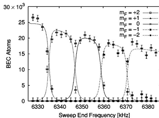
FIG. 3. Final population of  $m_F$  states after a Landau-Zener sweep starting at 6326 kHz vs sweep end frequency. The horizontal errors represent the accuracy of the used sweeping generator. A theoretical model is fitted to the data to determine a magnetic-field calibration yielding a linear Zeeman splitting frequency of  $2\pi \times (6353.13 \pm 0.08)$  kHz.
