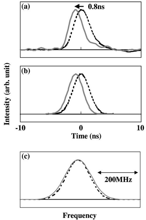
FIG. 7. (a) Observed negative delay of the probe pulse (solid line) in the anomalous dispersion region for the atomic density of  $9.3 \times 10^{11} \text{ cm}^{-3}$  [ $78^\circ\text{C}$ , Fig. 5(c)]. The broken line is zero delay for off-resonance. (b) Simulation of (a) calculated from Eq. (9). (c) Simulation of incident (broken line) and transmitted (solid line) spectra.
