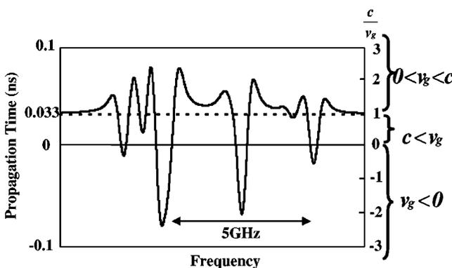
FIG. 2. Simulation of the propagation time for a 1 cm Rb cell of Fig. 1 ( $45^\circ\text{C}$ ). The broken line indicates the propagation time (33 ps) for  $c$ , light velocity in vacuum.
