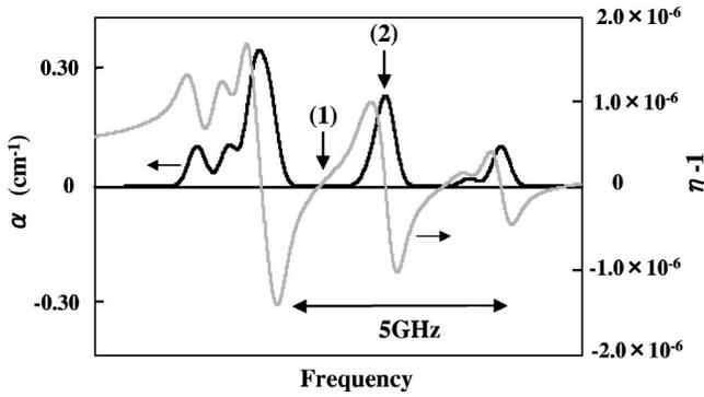
FIG. 1. Absorption coefficient  $\alpha$  and change  $\eta-1$  of the refractive index of the Rb  $D_1$  transition for the atomic density of  $6.5 \times 10^{10} \text{ cm}^{-3}$  ( $45^\circ\text{C}$ ). Arrows (1) and (2) indicate the frequency of the probe pulse.
