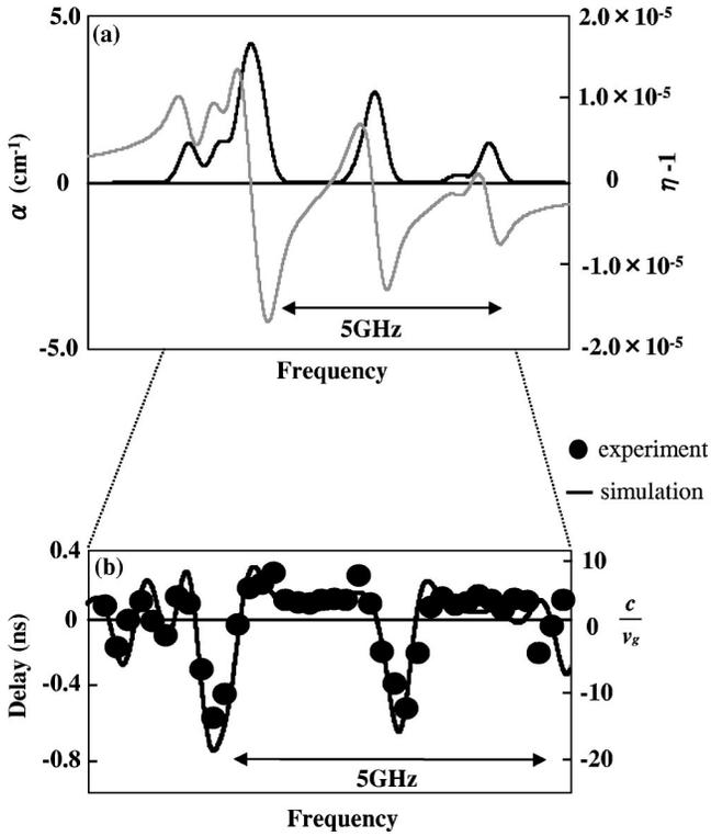
FIG. 8. (a) Absorption coefficient  $\alpha$  and change  $\eta-1$  of the refractive index for the atomic density of  $4.5 \times 10^{11} \text{ cm}^{-3}$  ( $65^\circ \text{C}$ ). (b) Frequency dependence of the delay time of the probe pulse (solid circles). The solid line is a theoretical curve calculated by applying  $d\omega/dk$  of Eq. (5).
