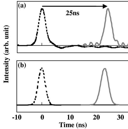
FIG. 6. (a) Observed delay of the probe pulse (solid line) in the normal dispersion region for the atomic density of  $2.3 \times 10^{14} \text{ cm}^{-3}$  [ $175^\circ\text{C}$ , Fig. 4(c)]. The broken line is zero delay for off-resonance. (b) Simulation of (a) calculated from Eq. (9).
